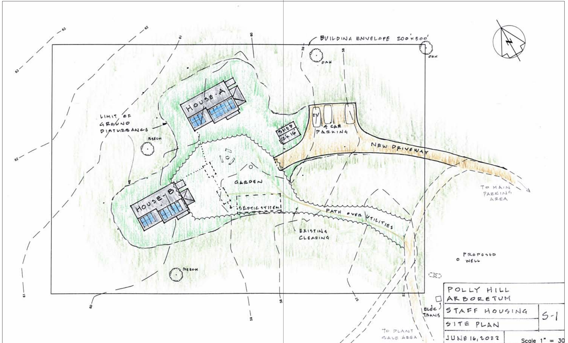
Figure 3 Building Envelope and Site Plan
